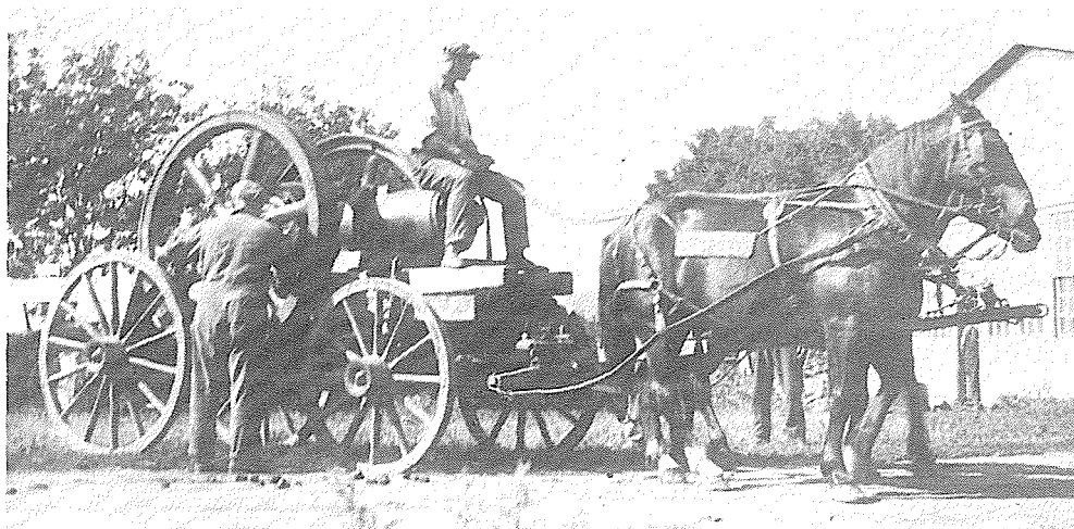
Bringing a hit and miss gas engine to Friesen's light plant, probably in 1911. This engine proved to be inadequate within five years and was replaced by a 15 h.p. diesel.
